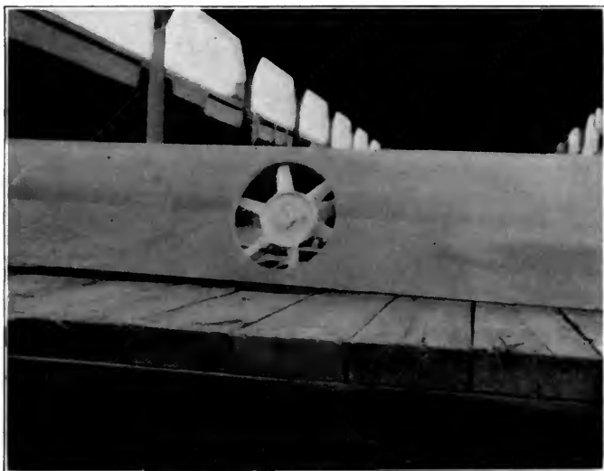
FIG. 5.—ELECTRICAL FAN MOUNTED ON A BOARD READY FOR INSTALLATION IN A REFRIGERATOR CAR
